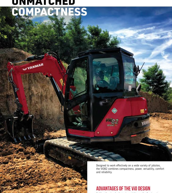
Neither the standard counterweight, nor the front part of the upper frame sticks out of the track width. With this being a true zero tail swing excavator the ViO82 provides the best conditions for working safely and comfortable on any working site with limited space.
