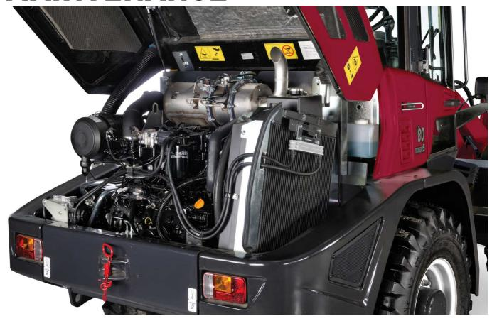
The large opening offered by the engine hood allows an easy access to all main service items, for an easy and fast maintenance. This contributes to reduce the total cost of ownership (TCO) of the machine. Daily tasks can be performed from ground level to save time.
